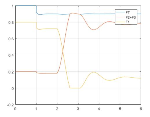
The total feed rate, FT, and the sum of feed rates F2 and F3 coincide for  $1.7 \le \tau \le 2.2$ . If the custom input constraints had not been included, the controller would have requested an impossible negative feed 1 rate, F1, during this period.
