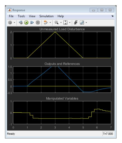
The plant input and output signals are identical to those obtained using the built-in Model Predictive Control Toolbox solver, but the qp.status shows that quadprog does not take the same number of iterations to find a solution. However, it does detect the same infeasibility time period. bdclose(mdl);
