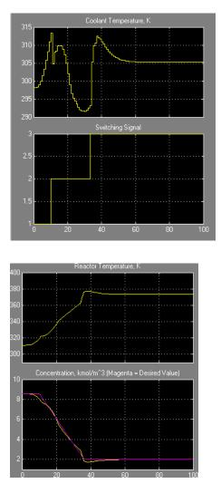
The above plots show the simulation results. The Multi MPC Controller block uses the three controllers sequentially as expected (see the switching signal). Tracking of the concentration setpoint is excellent and the reactor temperature is also controlled well.
