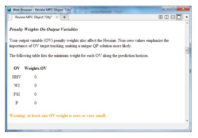
The review has flagged the zero weights on all four output variables. Since the zero weights are consistent with the design requirement and the other Hessian tests indicate that the quadratic programming problem has a unique solution, this warning can be ignored.
