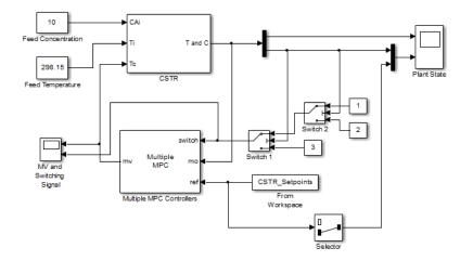
The two CSTR outputs are the reactor temperature and composition respectively. These are being sent to a scope display and to the control system as feedback.
