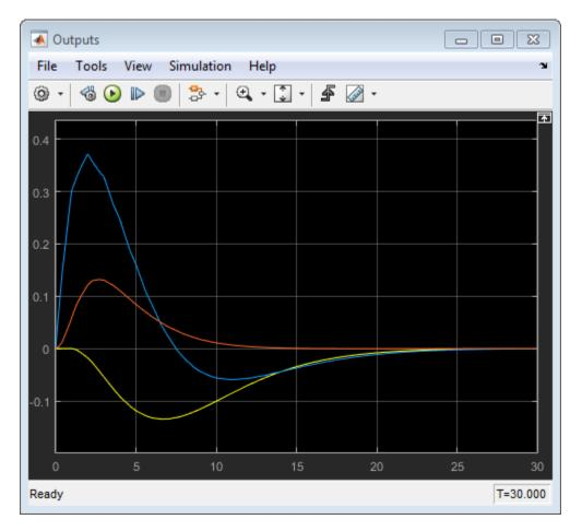
In the **Outputs** plot, the responses are almost identical to the responses from the corresponding simulation in MPC Designer. The yellow curve is  $H_2$ , the blue is  $N_1$ , and the red is  $N_2$ .
