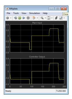
For the first 90 time units, the Switching Signal is 0, which makes the system operate in automatic mode. During this time, the controller smoothly drives the controlled plant output from its initial value, 0, to the desired reference value, -0.5.
