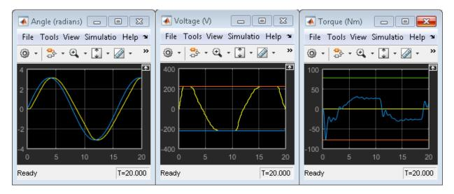
In the **Angle** scope, the output response, yellow, tracks the angular position setpoint, blue, closely.
