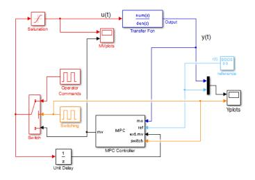
To simulate switching between manual and automatic operation, the Switching block sends either 1 or 0 to control a switch. When it sends 0, the system is in automatic mode, and the output from the MPC Controller block goes to the plant. Otherwise, the system is in manual mode, and the signal from the Operator Commands block goes to the plant.
