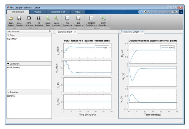
The initial design uses a conservative control effort to produce a robust controller. The response time for output  $H_2$  is about 7 minutes. To reduce this response time, you can decrease the sample time, reduce the manipulated variable rate weights, or reduce the manipulated variable rate constraints.
