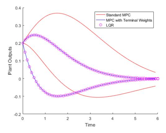
The plot shows that the MPC controller with the terminal weights provides faster settling to the origin than the standard MPC. The LQR controller and MPC with terminal weights provide identical control performance.
