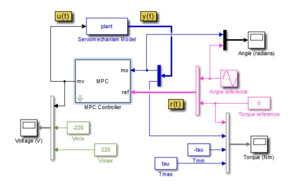
This model uses an MPC Controller block to control a servomechanism plant. The Servomechanism Model block is already configured to use the plant model from the MATLAB workspace.
