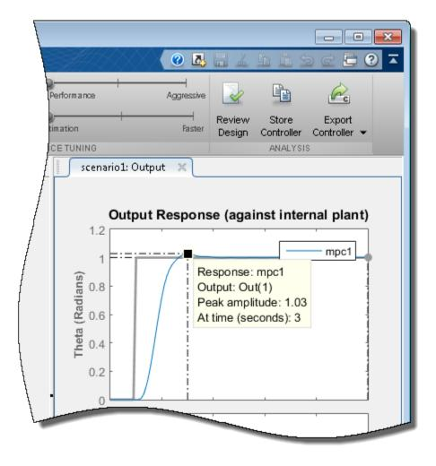
The peak output response occurs at time of 3 seconds with a maximum overshoot of 3%. Since the reference signal step change is at 1 second, the controller has a peak time of 2 seconds.
