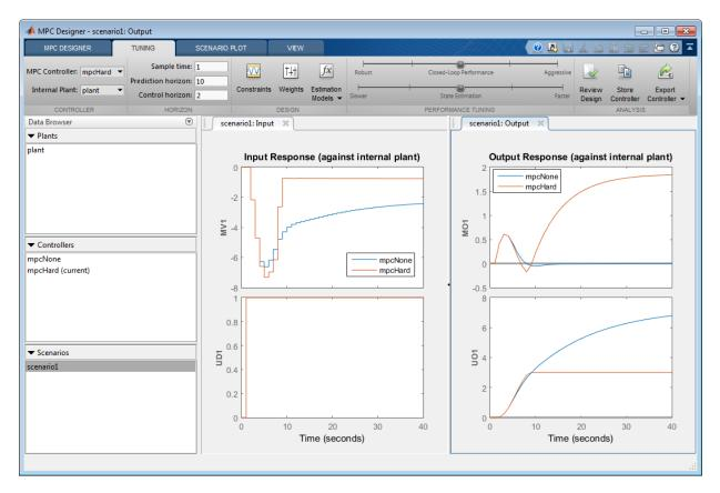
The response plots update to reflect the new mpcHard configuration. In the **Output Response** plot, in the **UO1** plot, the mpcHard response is limited to a maximum of **3**. As a trade-off, the controller cannot return the **MO1** response to its nominal value.
