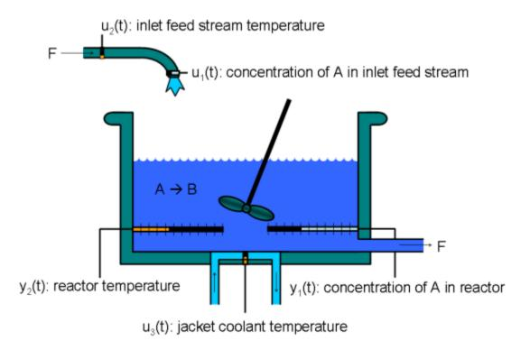
This is a jacketed non-adiabatic tank reactor described extensively in Seborg's book, "Process Dynamics and Control", published by Wiley, 2004. The vessel is assumed to be perfectly mixed, and a single first-order exothermic and irreversible reaction, A --> B, takes place. The inlet stream of reagent A is fed to the tank at a constant volumetric rate. The product stream exits continuously at the same volumetric rate and liquid density is constant. Thus the volume of reacting liquid is constant.
