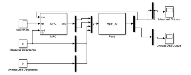
The app exports the current MPC controller and its internal plant model to the MATLAB workspace and creates a Simulink model that contains an MPC Controller block and a Plant block
