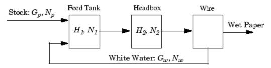
The process is nonlinear and has three outputs, two manipulated inputs, and two disturbance inputs, one of which is measured for feedforward control.
