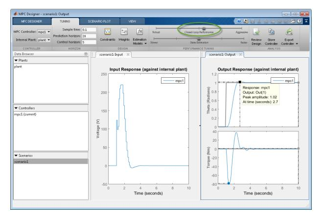
The final controller peak time is 1.7 seconds. Reducing the response time further results in overly-aggressive input voltage changes.
