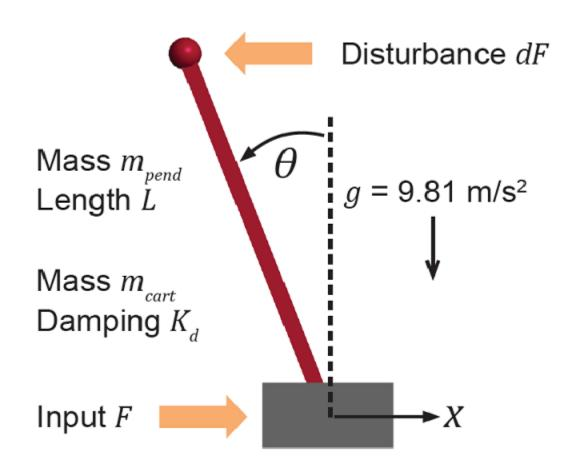
This system is controlled by exerting a variable force F on the cart. The controller needs to keep the pendulum upright while moving the cart to a new position or when the pendulum is nudged forward by an impulse disturbance dF applied at the upper end of the inverted pendulum.
