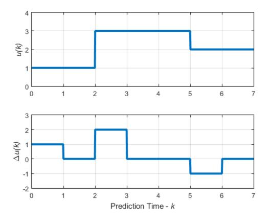
Blocking Moves: Inputs and Input Increments for moves = [2 3 2]
