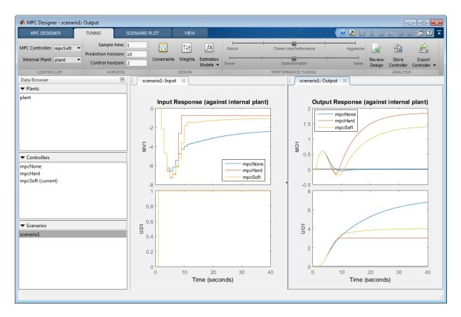
The response plots update to reflect the new mpcSoft configuration. In the **Output Response** plot, mpcSoft shows a compromise between the previous controller responses.
