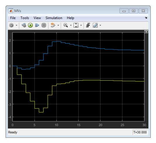
The mismatch between the prediction model and the plant now produces output responses with significant differences. Increasing the disturbance magnitude further results in large setpoint deviations and saturated manipulated variables.
