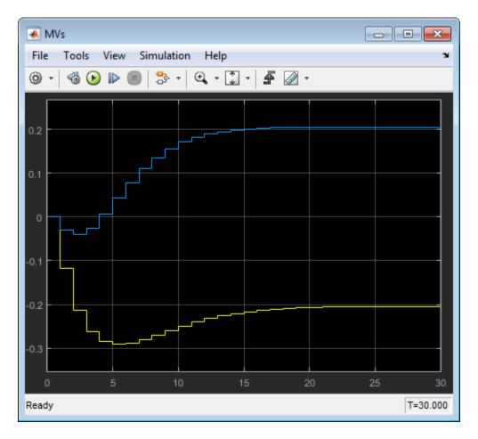
Similarly, in the **MVs** scope, the manipulated variable moves are almost identical to the moves from corresponding simulation in MPC Designer. The yellow curve is  $G_p$  and the blue is  $G_w$ .
