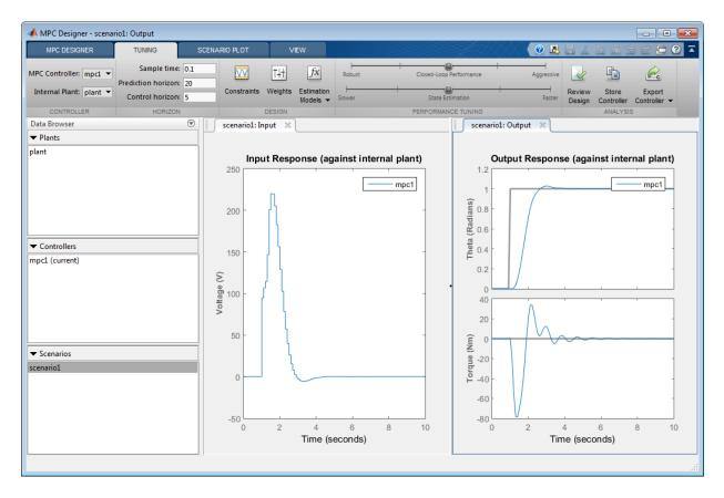
The response plots update to reflect the increased rate weight. The **Input Response** is smoother with smaller voltage changes.
