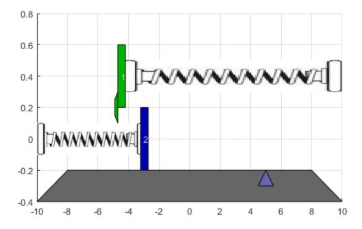
In this case, performance degrades when the masses separate, causing the controller to apply excessive force.
