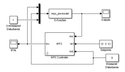
TheMPC Controller block controls the nonlinear paper machine plant model, which is defined using the S-Function mpc\_pmmodel.
