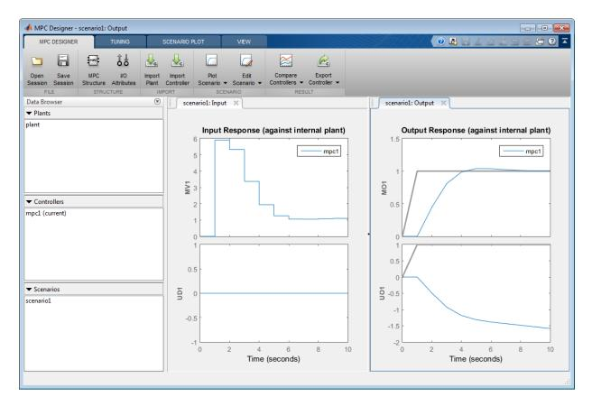
The app adds the specified plant to the **Data Browser** along with a default controller, mpc1, and a default simulation scenario, scenario1.
