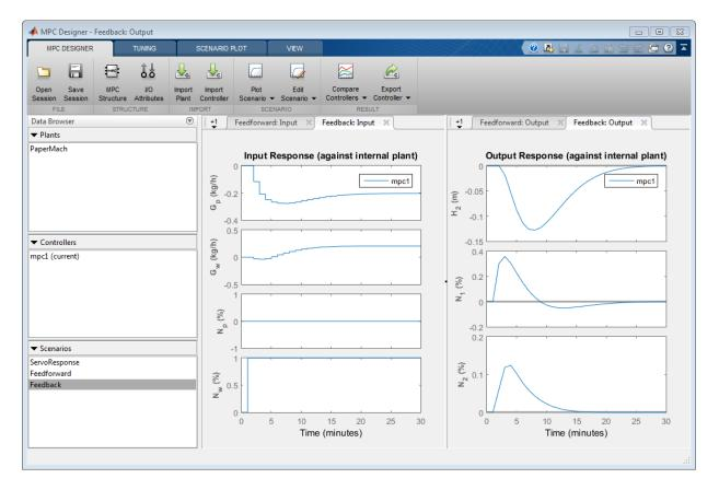
The controlled outputs,  $H_2$  and  $N_2$ , both exhibit relatively small deviations from their setpoints. The settling time is longer than for the original servo response, which is typical.
