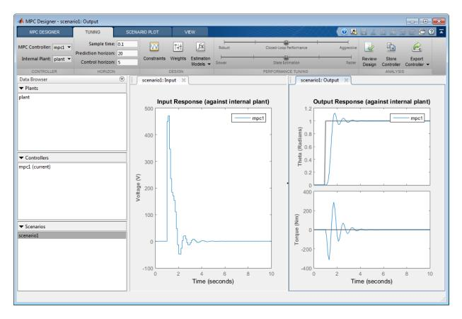
As you update the sample time and horizon values, the **Input Response** and **Output Response** plots update automatically. Both the input voltage and torque values exceed the constraints defined in the system model specifications.
