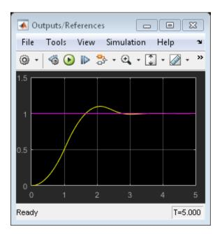
Simulate with Explicit MPC controller in Simulink. Controller "mpcobjExplicitSimplified" is specified in the block dialog.
