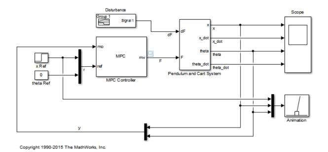
Although cart velocity  $x\_dot$  and pendulum angular velocity *theta\\_dot* are available from the plant model, to make the design case more realistic, they are excluded as MPC measurements.
