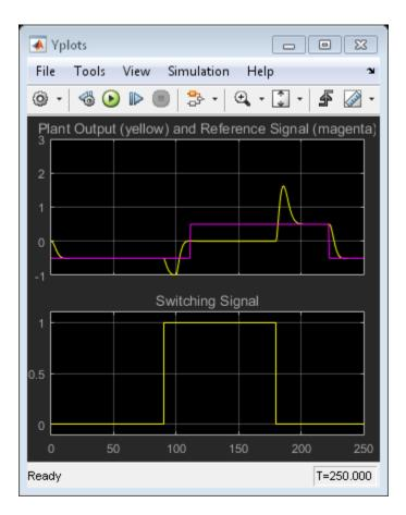
Now the transition from manual to automatic control is much less smooth. Note the large "bump" between time = 180 and 200.
