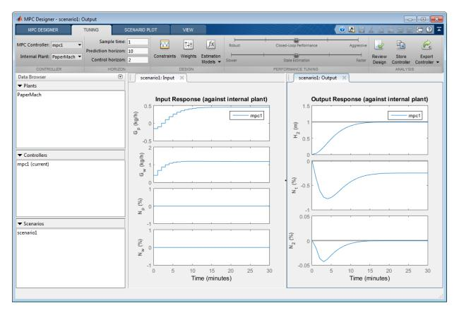
The controller places more emphasis on eliminating errors in feed tank consistency,  $N_2$ , which significantly decreases the peak absolute error. The trade-off is a longer response time of about 17 minutes for the feed tank level,  $H_2$ .
