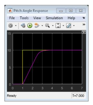
The closed-loop response is identical to the traditional MPC controller designed in the "mpcaircraft" example.
