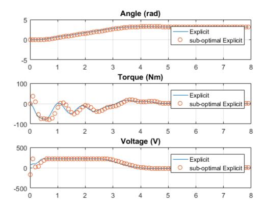
The simulation result with the sub-optimal Explicit MPC is slightly worse. bdclose(mdl)
