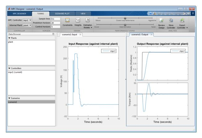
The response plots update to reflect the new constraints. In the **Input Response** plot, there are undesirable large changes in the input voltage.
