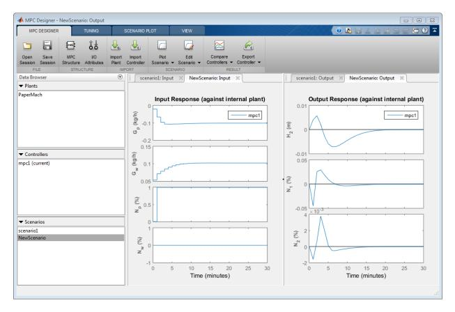
The manipulated variables begin changing before the measured disturbance occurs because the controller uses the known future disturbance value when computing its control action. The output disturbance values also begin changing before the disturbance occurs, which reduces the magnitude of the output errors. However, there is no significant improvement over the previous simulation result.
