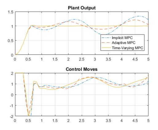
Only the time-varying MPC controller is able to bring the plant output close enough to the desired setpoint.
